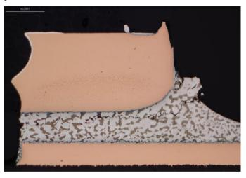
Fig. 7. Cross-section of SnPb soldered QFN component with 12 ppm/°C mold compound and non-wettable flanks
