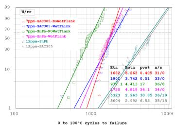
Fig. 4. Weibull distribution of 6 tested QFN64 solder assemblies.
