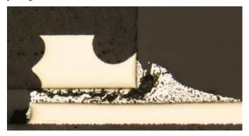
Fig. 6. Cross-section of SnPb soldered QFN component with 7 ppm/°C mold compound and wettable flanks
