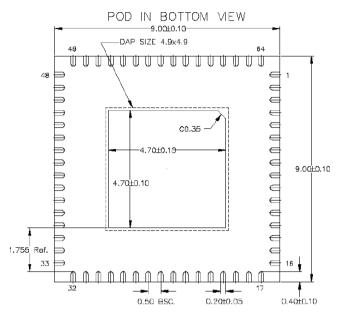
Fig. 2. Package outline drawing for the QFN package used in this BLR analysis
