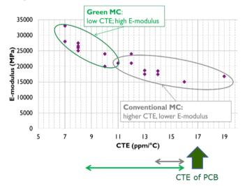
Fig. 1. Correlation between the mold CTE and mold stiffness for a wide range of commercially available mold compounds. The graph also indicates the larger gap between the CTE's of the PCB and the green mold compounds
