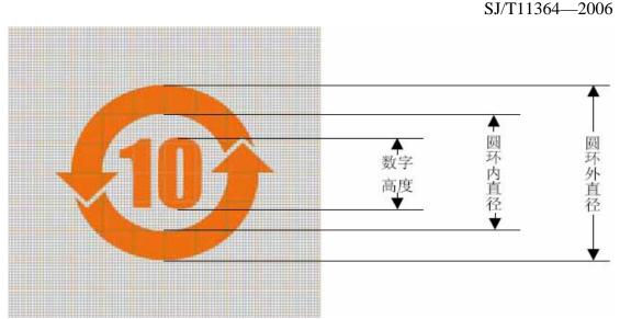
[Chinese characters in Figure translated as follows, left to right: "height of numbers," "inner diameter," "external diameter"] Figure 4
